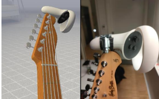
Figure 5: The virtual setup (left) and the physical setup (right) of the left-hand controller attached to the guitar head.
